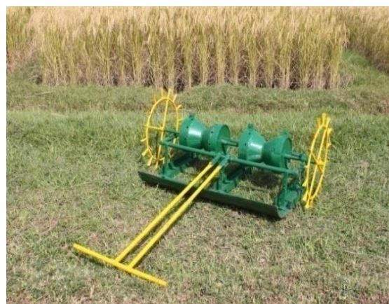
Four row manual drum seeder
