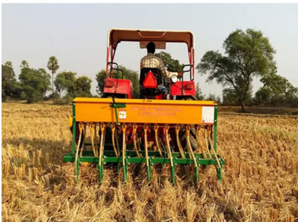
2) Sowing of wheat with Happy Seeder in Rice residue
