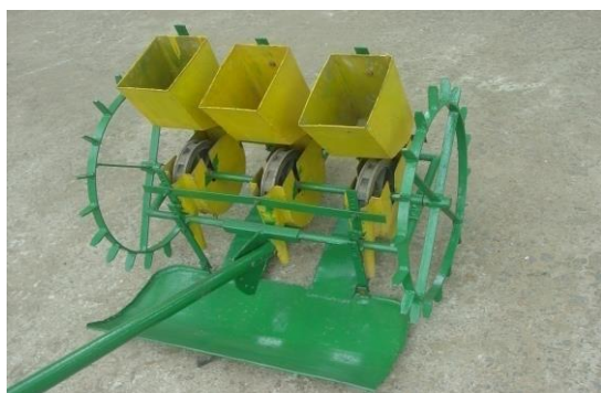
Three row manual puddle seeder
